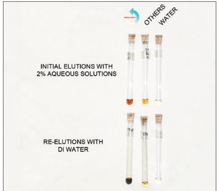
Picture above shows elutant collection of 2% solutions of REVERT compared to OARS and water (control). Color difference is result of humic substance contaminant removal from the soil.
