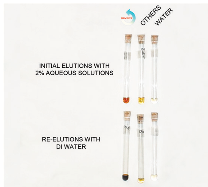
Picture above shows elutant collection of 2% solutions of REVERT compared to OARS and water (control). Color difference is result of humic substance contaminant removal from the soil.
