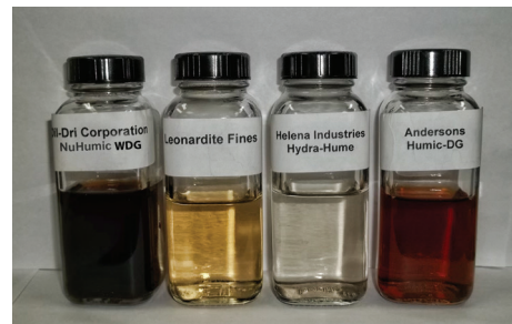
Darker brown color of NuHumic WDG sample indicates a higher percentage of soluble humic acids in water extract.
